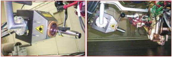
Figure 6 – Commercially available 4 kW Direct diode laser and IR pyrometer mounted on a fiber placement head.
