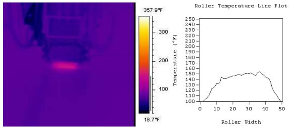
Figure 7. IR image of the resulting heat from a diode laser illumination of nit-point between substrate and incoming tow prepreg.
