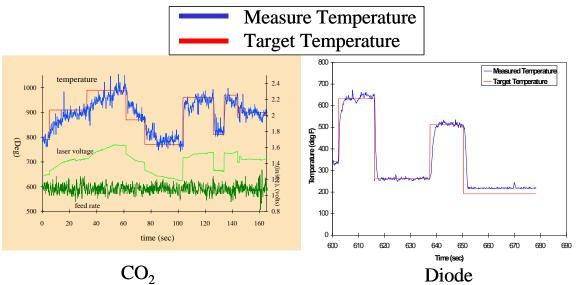
Figure 4 – Temperature Comparison of CO<sub>2</sub> and Diode laser heater
