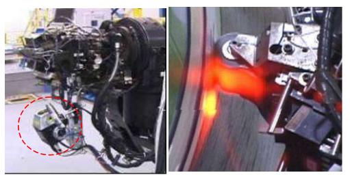
Figure 9: GKN's Ingersoll placement head and detail of compaction region during placement. The laser (black box) and pyrometer (cylinder) are circled in the first photo, and the resulting thermal image is shown in the second. [11]
